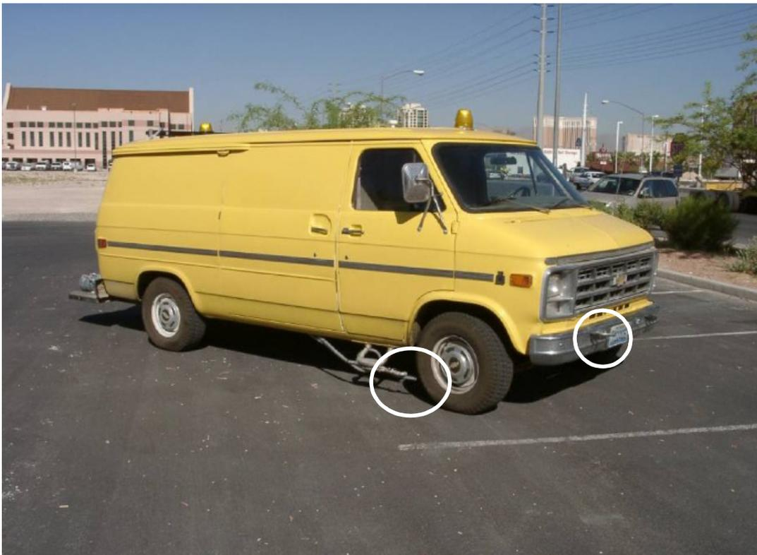
The TRAKER II inlet lines are configured so that on unpaved roads, where  $PM_{10}$  concentrations behind the front tires could exceed the particle monitor upper limit ( $150 \text{ mg/m}^3$ ), clean air can be mixed with air from the wheel well inlets in a controlled manner to achieve a
