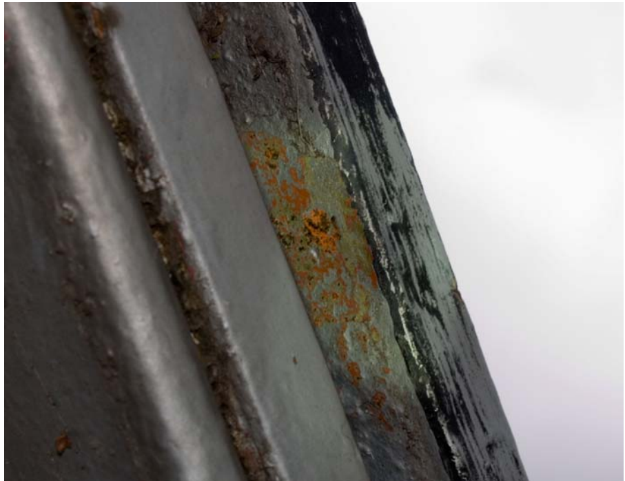
Black, orange, green and aluminum layers on back of plaque
