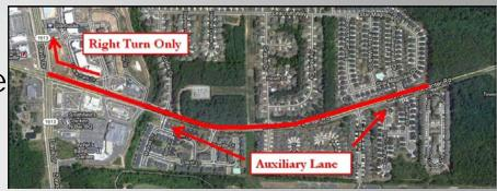
4,500-ft lane between two interchange ramps and ending in turn lane, proposed for safer weaving
