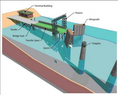
Key parts of a typical ferry terminal
