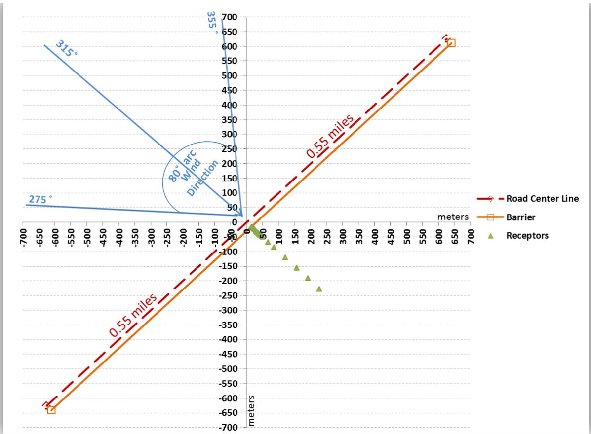
Figure 2. Aerial view illustrating the configuration of the modeled roadway and predominant wind direction relative to the barrier and receptors.
